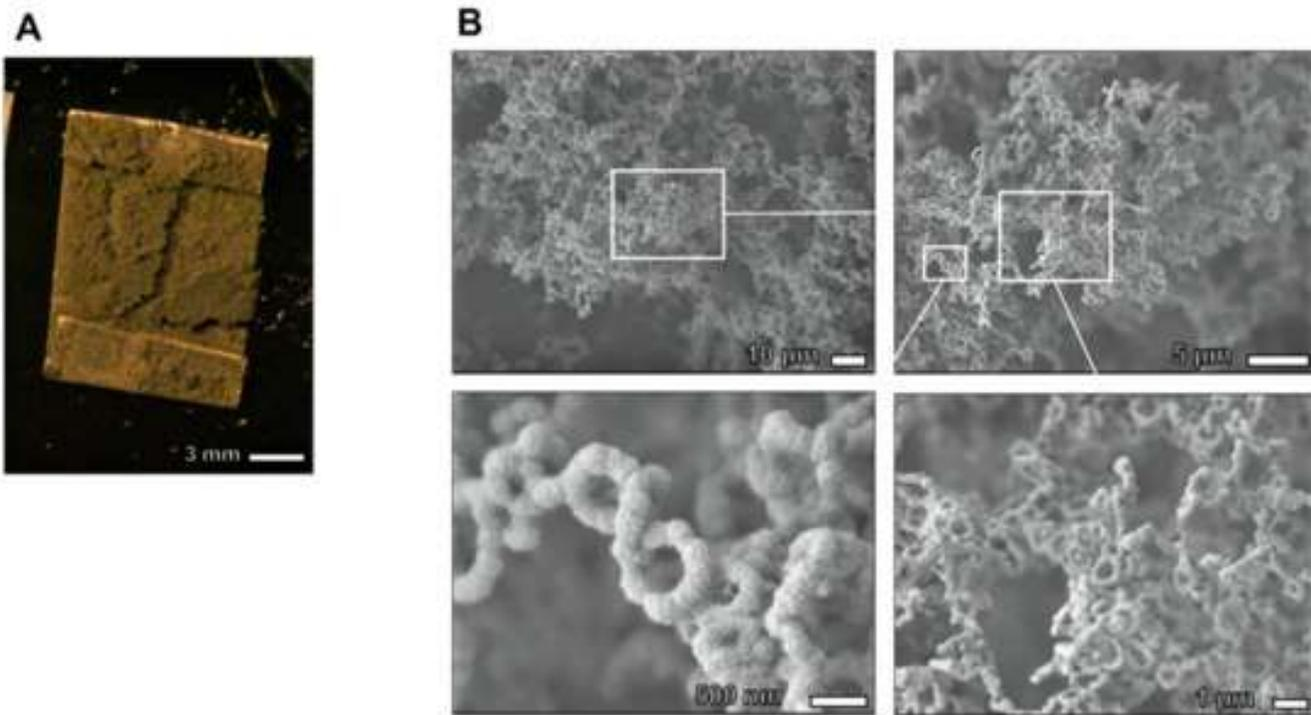
fabrication of 3D nanostructure using critical point drying method.
